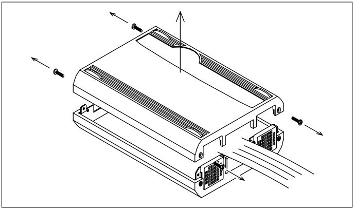
Figure 2.18 Removing the upper cover
